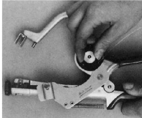
2. Push in knurled nut and then tighten until the reel is **lightly braked**.
