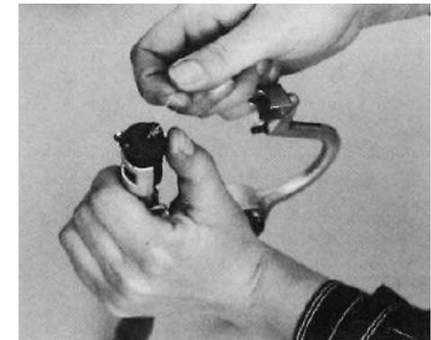
8. ... or remove it in the direction of the press-in device by pressing on the wire retainer.
